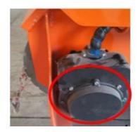
②Screw the M6\*25 bolt into the screw holes in the brake disc, see Figure2;
