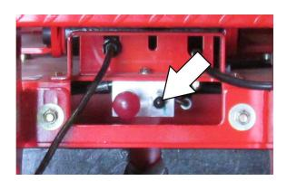
4) Pull the red brake release pump knob.
